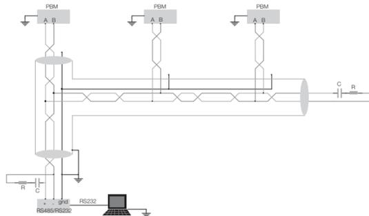
The relay PBM B has a RS485 port to communicate with a remote computer or a SCADA system on a continuous basis. The protocol used is Modbus RTU (19200 -8 bit - no parity - 1 stop bit).
