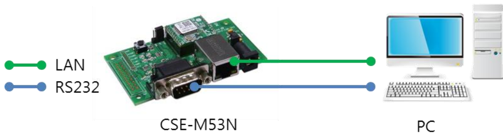
Figure 2-1 connection between CSE-M53N and a PC
