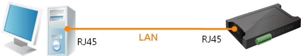
Figure 2-1 the connection between CIE-H14 and a PC
