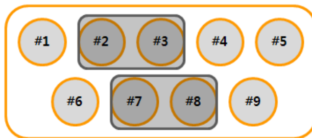
Fig 2-4 a D-sub 9 pin RS232 Loopback connector
