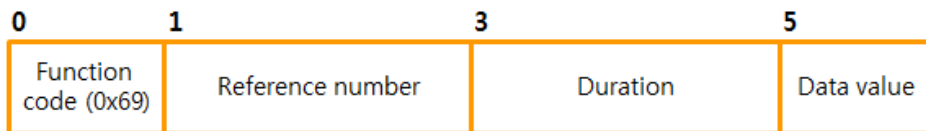
Figure 3-1 request / response frame of the Write Pulse
