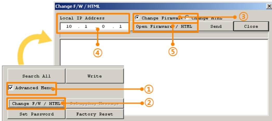
Fig 2-3 running TFTP client
