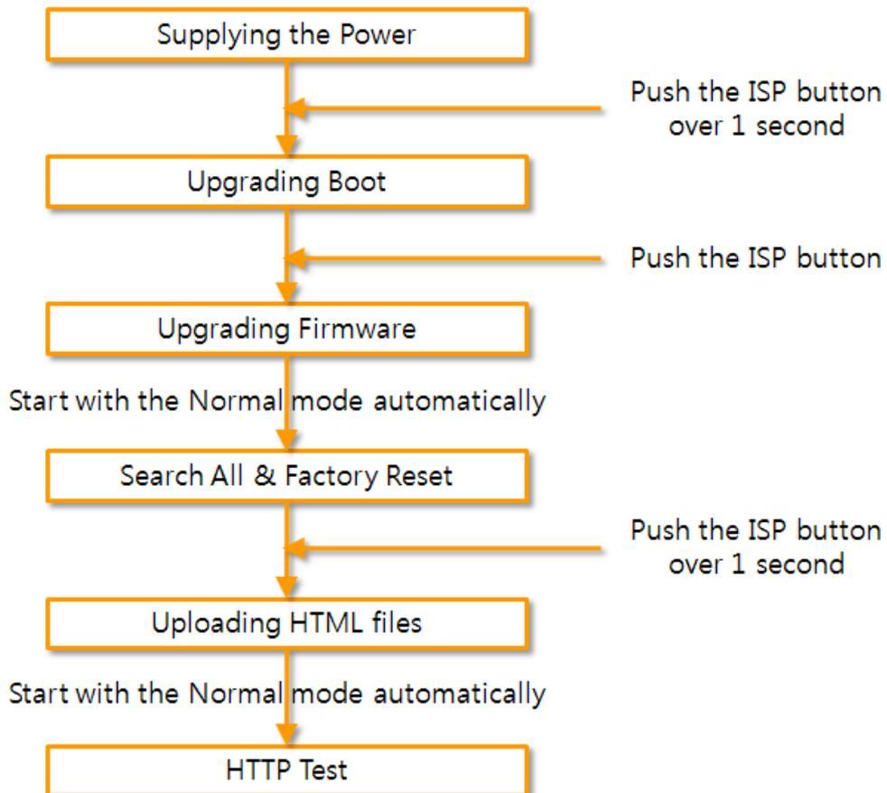
Fig 2-1 Diagram for upgrading boot and firmware
